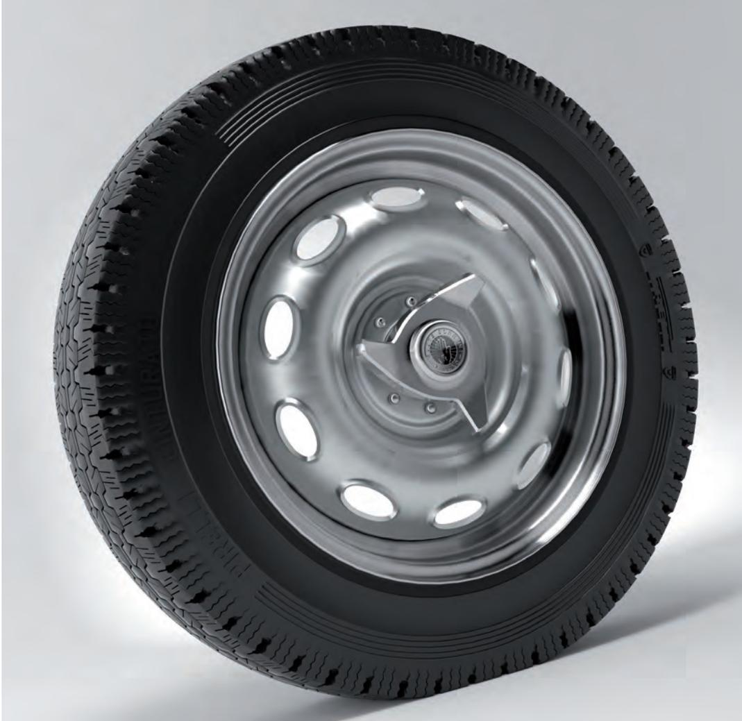
*The R1-257 has a 4.50"x15" rim, ET 38 mm and 4 x 4.25" bolt pattern, and is available with Borrani silver painted centre and polished alloy rim as standard finish. This wheel is suitable for every model of Giulia and Giulietta with both disc or drum brakes. IMPORTANT: the "Turbo Sprint" centre lock wheel (shown in the picture) is supplied with integral Rudge type splined front hubs, the installation of these will require complete disassembly of the front brake system.*
